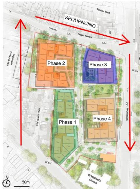
Figure 10.4.1 Indicative construction sequence for the LBH Civic Centre Site.
